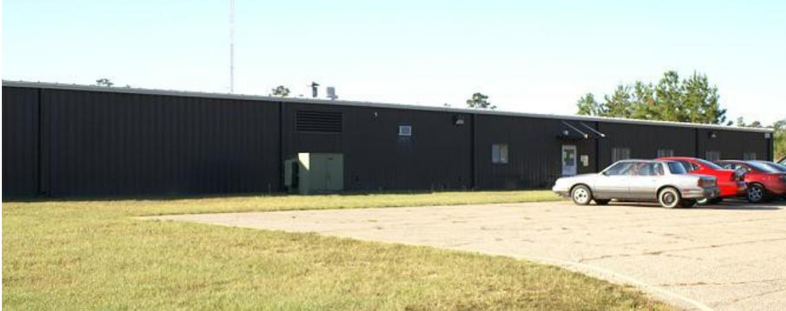
50,000 SF metal building consisting of 30,000 SF production/warehouse area, 6,700 SF production or warehouse area, 3,300 SF office/conference area, (all with HVAC) and 10,000 SF heated warehouse. The finished 150 x 200 manufacturing area has three rows of interior columns with 33 x 50 bays.
